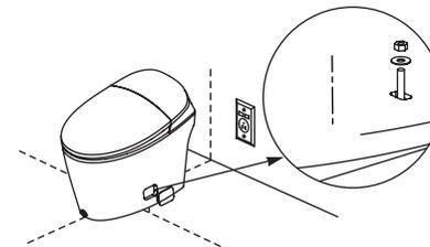
3. Secure the toilet base. Press down evenly on the toilet to set the wax ring. Install a washer and nut onto each bolt. Hand tighten the nuts. Use a wrench to tighten the nuts one quarter turn beyond hand tight.
