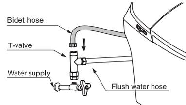
2. Attach the bidet hose to the T-valve and DLX.
