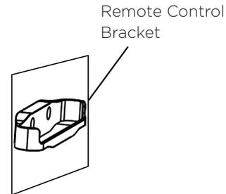
3. Place the remote bracket over the wall anchors.
