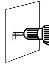
1. Drill two 6mm holes on the wall that line up with the remote bracket.
