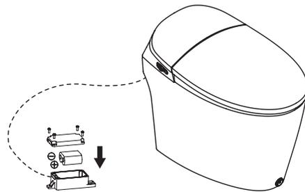
The battery should be kept out of children's reach. Please ensure that the battery's polarity is correctly matched. If they are incorrect it may lead to chemical leaks or explosions. The battery box is water proof so please make sure all the screws are tightly secured to ensure that the box is perfectly sealed.
