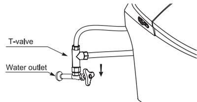
3. Connect the T-Valve to the water supply valve.
