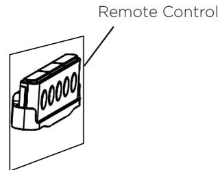
5. Place the remote control on the bracket.
