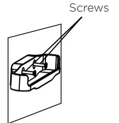
4. Use the provided screws to attach the remote control bracket to the wall.
