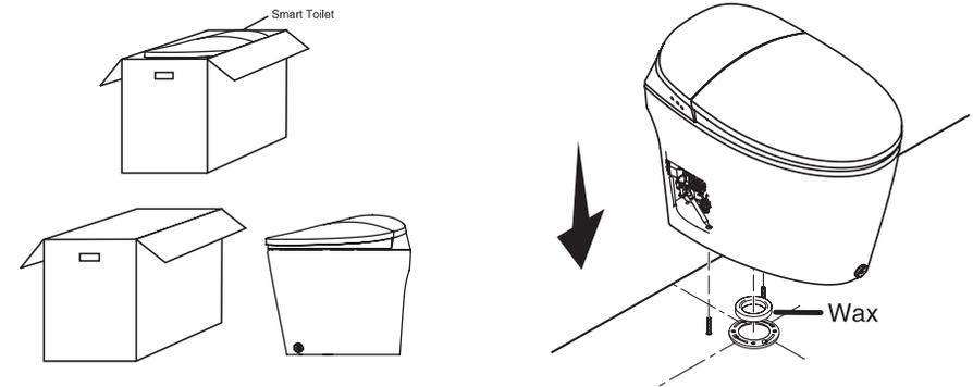
1. Open the box right side up. Remove the accessories first, then remove the unit from the top as shown in the diagrams above.
