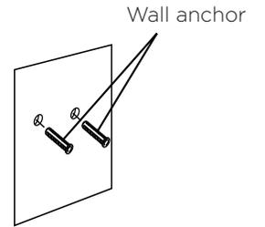
2. Install the wall anchors in the newly drilled holes.
