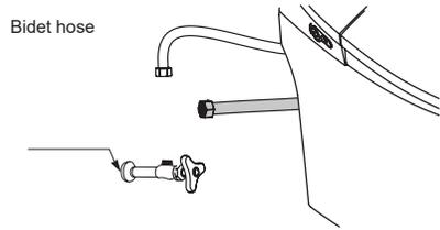
1. Attach the toilet hose to the T-valve and DLX.
