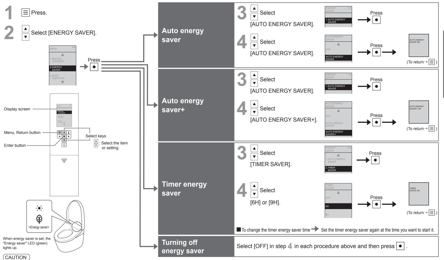
• During setting, the display goes out when no button is pressed within about 60 seconds. If you fail to complete the setting, redo from the step 1.
